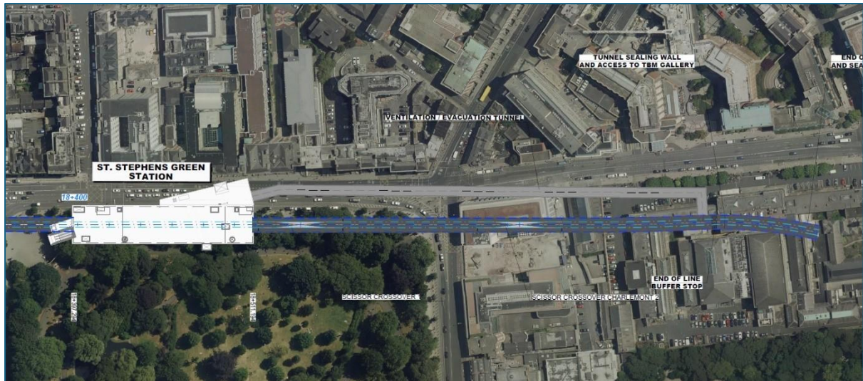
Figure 5: St Stephen's Green East as a terminus with evacuation/ventilation tunnel to the east
